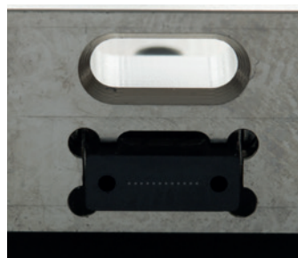
Close-up of the LightCONEX LC 12-lane plug-in module connector.
