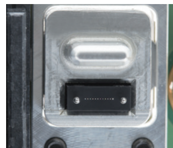
Close-up of the SpaceCONEX28 SC 4+4-lane backplane connector.
