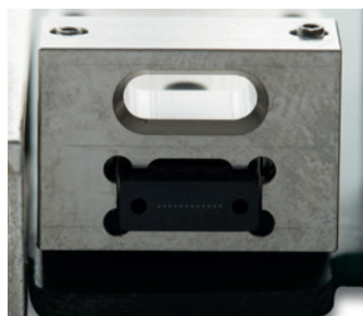
Close-up of the SpaceCONEX28 SC 4+4-lane plug-in module connector.
