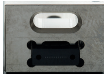
Close-up of the SpaceCONEX SC 12-lane plug-in module connector.
